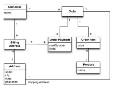
Figure 12: Data Model Oriented Around a Relational Database
