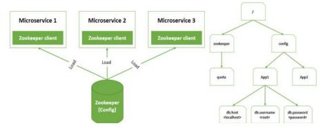
Figure 7 Zookeeper [Centralized configuration service]
